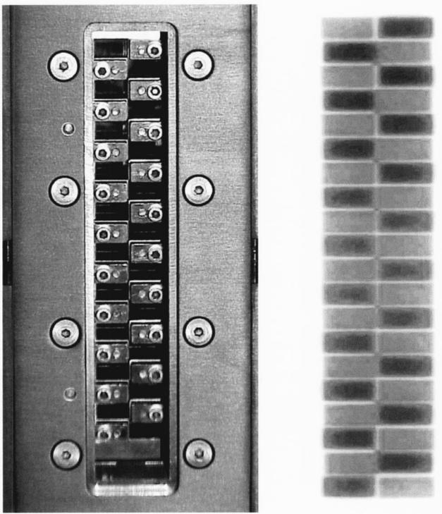
FIG. II.4. Checkerboard pattern design using MIMiC<sup>®</sup> leaves and the resulting exposed film from laterals. Reprinted with permission from Saw *et al.* (Ref. 27).
